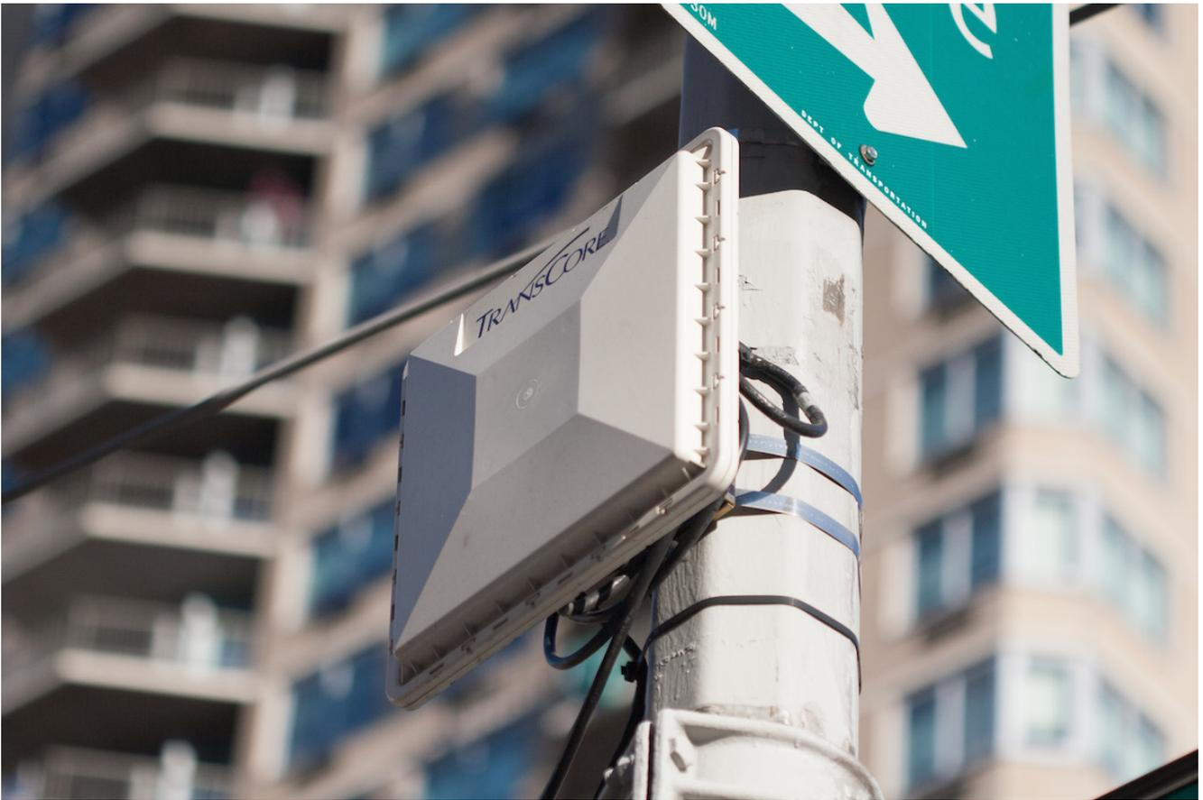
Figure 1: A typical roadside reader mount
