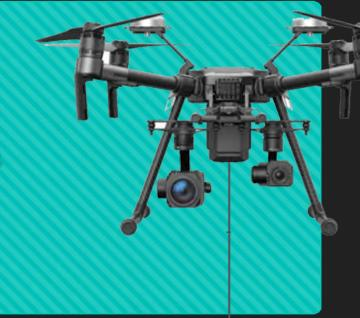
Powering both the drone and its sensors from the ground has a number of advantages. For one, flight time is extended from less than an hour (with most current UAS) to days. Additionally, a tether can supply more power than a battery, which means larger motors and heavier payloads.
